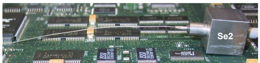
Whether the non-contacting infrared sensor or the K-type thermocouple is used depends on the soldering application.
