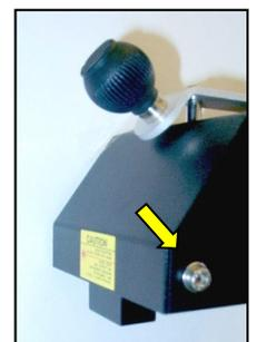
When the laser dot is adjusted properly it marks exactly the spot where the pipette contacts the board when pressed down.
